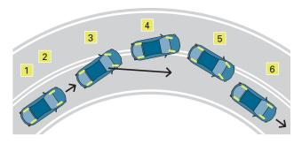
Front-wheel skids are caused by hard braking, acceleration or by driving too fast for the road conditions. You can't steer when the front wheels lose traction. To regain steering control:
