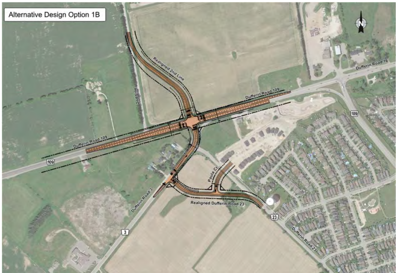
Figure 6-6: Option 1b: 2nd Line Amaranth Realignment (Dufferin County Road 23 Diverted to Dufferin County Road 3)
